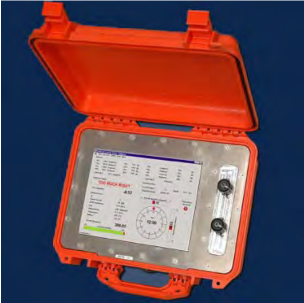
Figure 4. The display of the drilling engineer, which additional to the PC display of the surveyor. The drilling engineer pushes a button to let the software count for the number of pipes of known length. For RLG system the drilling machine cylinder stroke is measured to avoid human errors.
