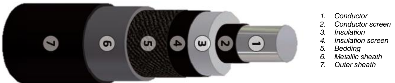
Figure 6 HVAC 220 kV land export cable
