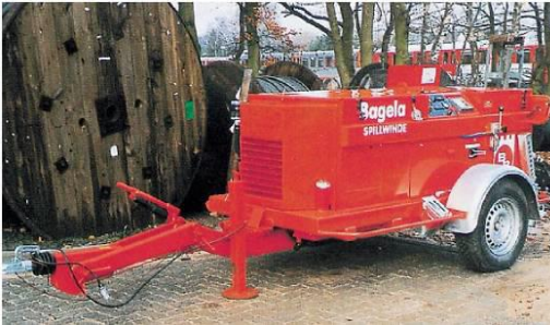
Figure 20 Typical cable winch
