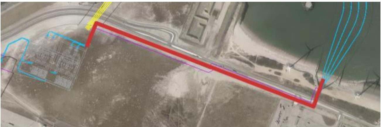
Figure 12 Onshore 220 kV export cable route
