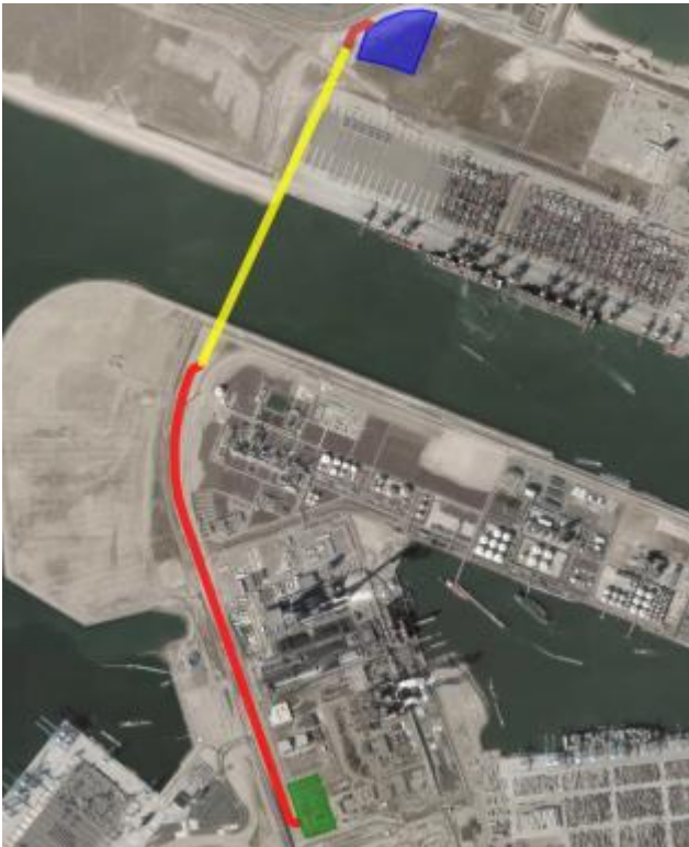
Figure 13 Onshore 380 kV cable route
