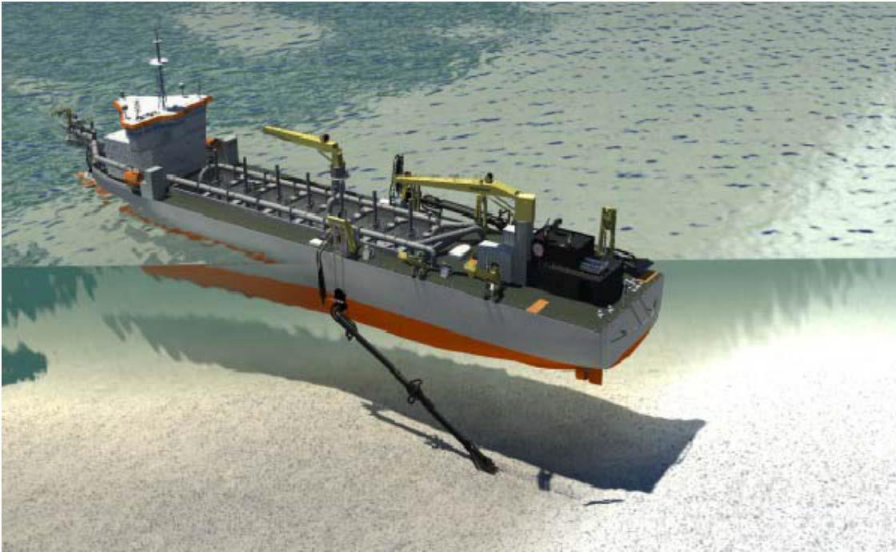
Figure 53 Trailing Suction Hopper Dredger
