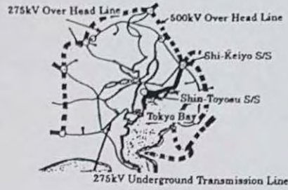
Fig.1- Cable route of Shinkeiyo-Toyosu Line
