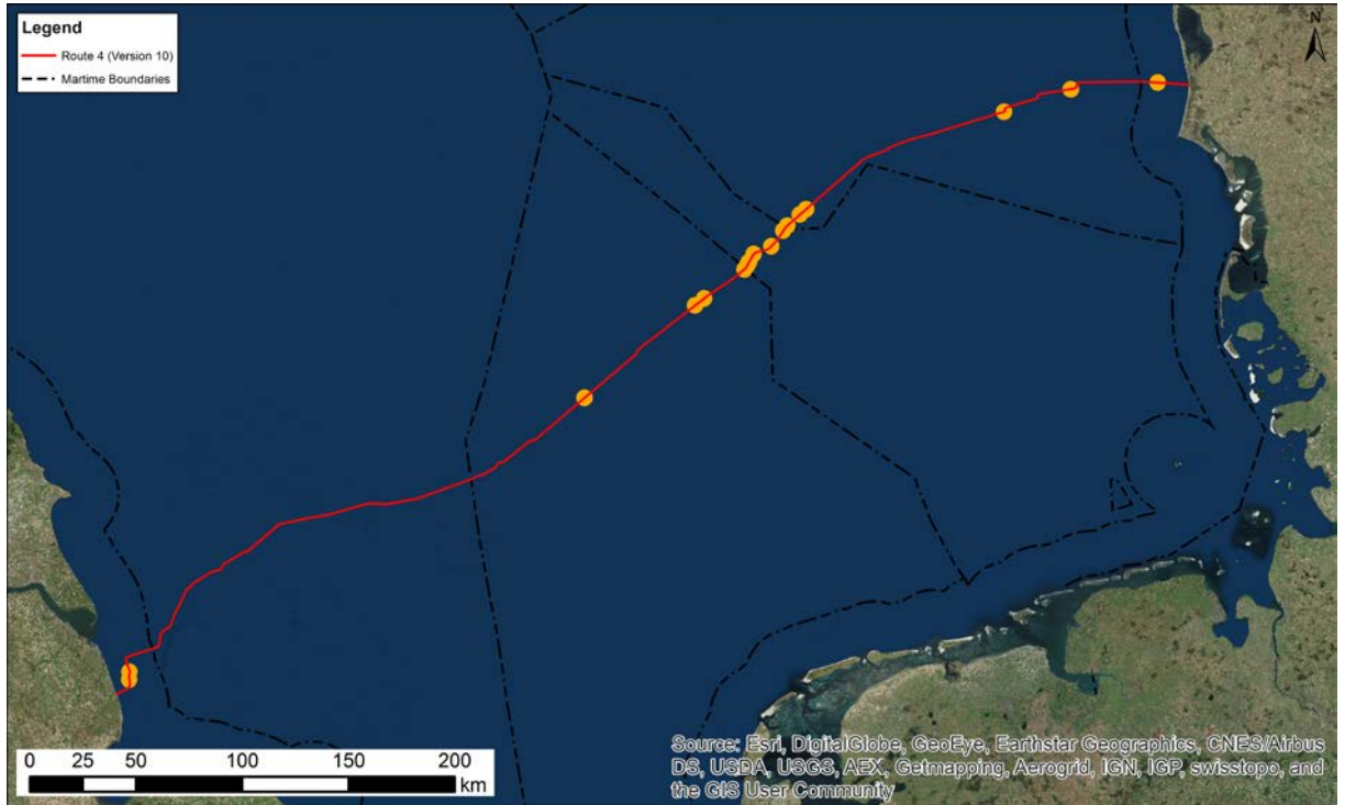
Figure 8.3: Occurrences of Peat along Route 4 (rev. 10), denoted as orange circles at 19 locations
