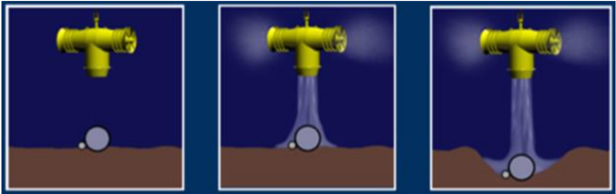
Figure 44 Mass flow excavation
