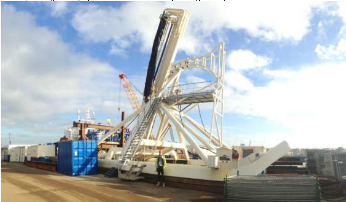
Figure 40 The BSS2 jet sledge
