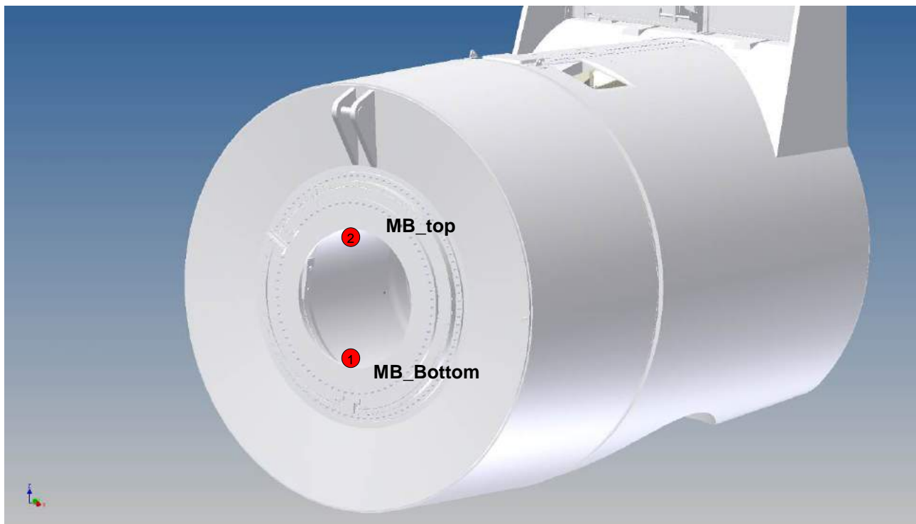
Figure 1: Measurement points on the main bearing.
