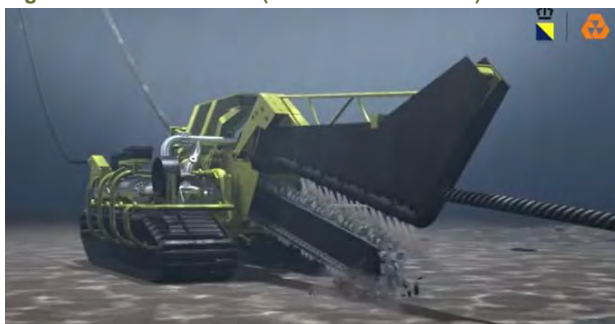
Figuur 2.12 Chain cutter (trench former VBMS)
