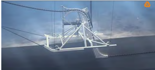
Figuur 2.13 Jetting tool (Burial sledge system VBMS)
