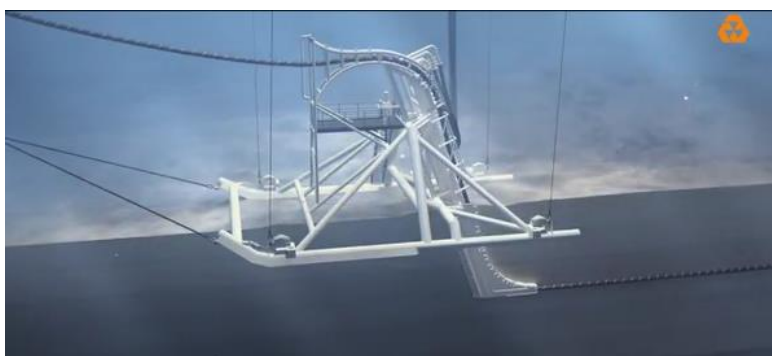
Figuur 1.34 Jetting tool (Burial sledge system VBMS)
