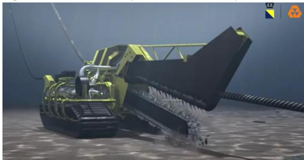
Figuur 1.33 Chain cutter (trench former VBMS)
